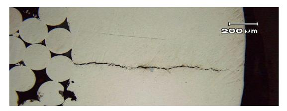
Figure 7 - Internal corrosion - flight control terminal sleeve.
