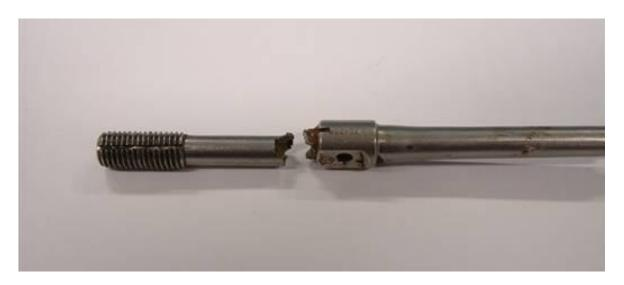
Figure 1 - Flight control cable terminal separation
