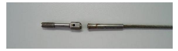
Figure 2 - Flight control cable terminal separation. Note that the failure has occurred outside the safety lockwire hole.
