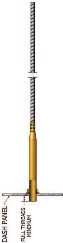
3. Carefully feed the inner wire into the housing and conduit, and thread the roller housing onto the brass housing while holding it. Tighten the lock washer and jam nut to secure the control to the dash panel. **Remember, the push rod must always remain engaged in the roller housing to avoid damage.**
