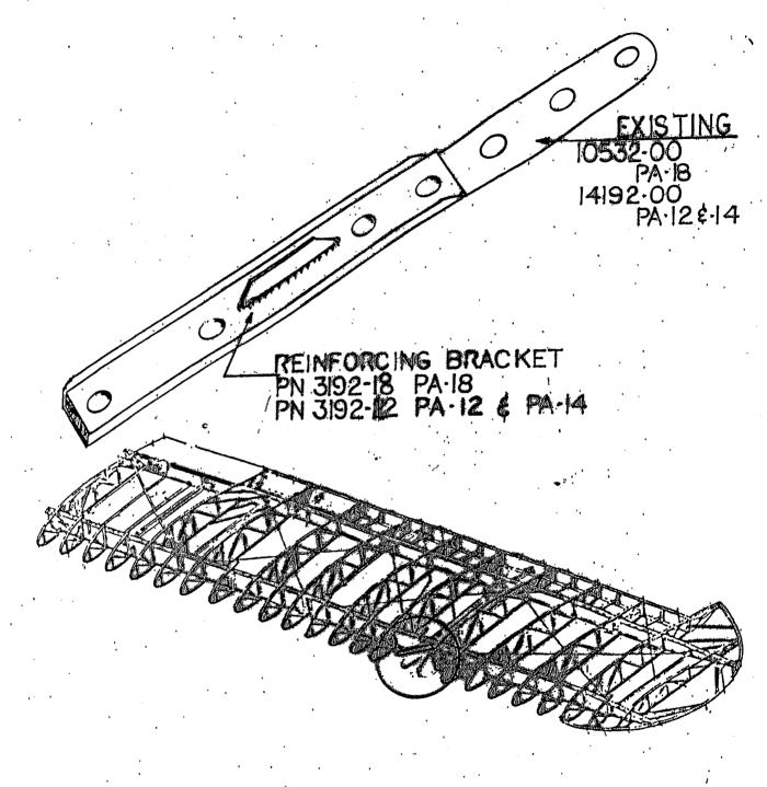
FRONT SPAR WING LIFT STRUT
