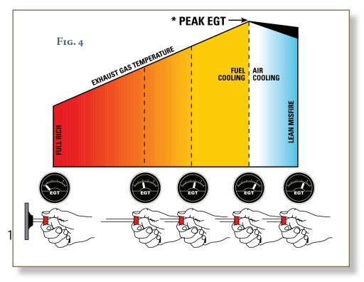
**REMEMBER:** When using the EGT method of mixture control, all mixture settings are made relative to peak EGT.
