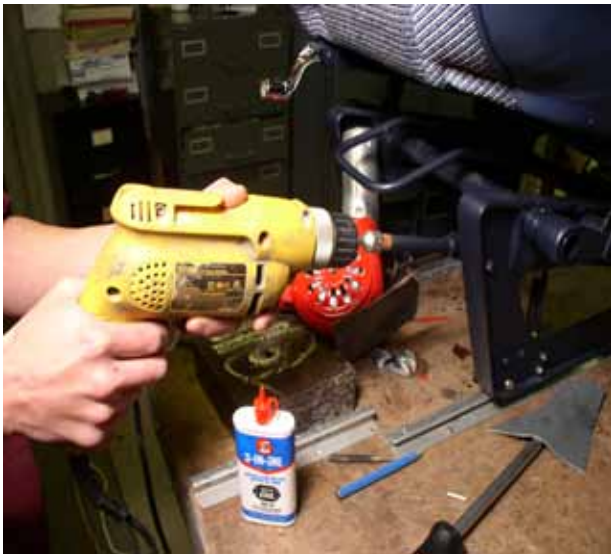
Drill motor trick to loosen tight seat height adjustment pivot shafts
