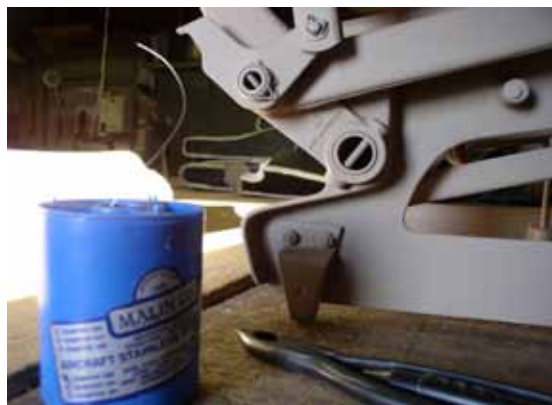
New roll pins installed and safety wired in the seat back reclining cam
