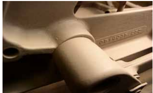
Seat height pivot points; definitely oil these at every annual inspection
