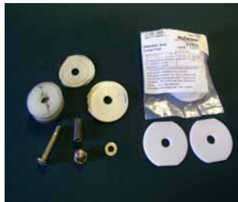
New McFarlane tefton thrust washers and seat rollers
