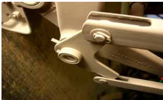
Loose roll pins halfway out of the seat back reclining bellcrank
