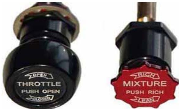
*Vernier Assist Throttle and Mixture Controls*
