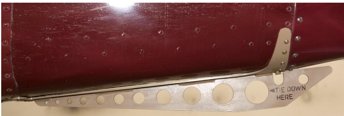
Figure 3-1, Replacement Tail Tie-Down Installation
